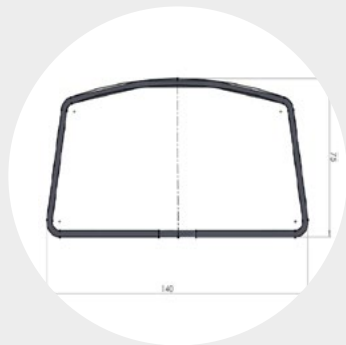
FRAME: CARBON STEEL 140 X 75 X 3 MM THICKNESS
